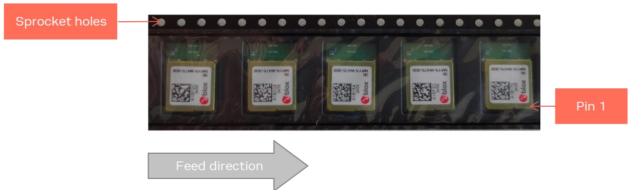
Figure 17: Orientation of MAYA-W4 modules on tape
