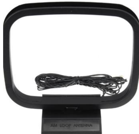
Figure 8 - Typical 'AM Air Loop' Antenna
