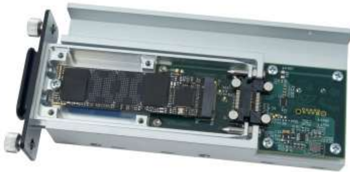
Removable drive shown installed in internal cradle
