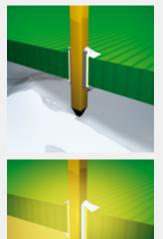
Solder pins are inserted into through-plated PCB holes and then soldered simultaneously using the wave soldering process.
